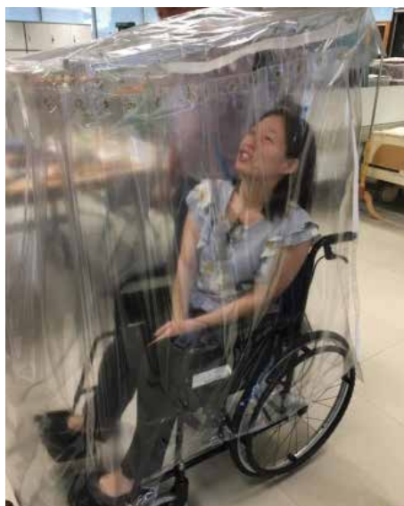
Prototype of wheelchair accessories designed by Ngee Ann Polytechnic Students – further refinement made to increase the protection for user
