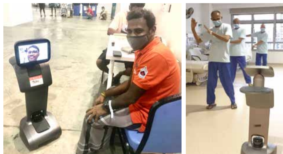
Temi can be deployed to patients' bedsides for non-urgent needs, act as a live translator for patients who speak different languages, deliver medications to patients, and facilitate tele-counselling sessions.
